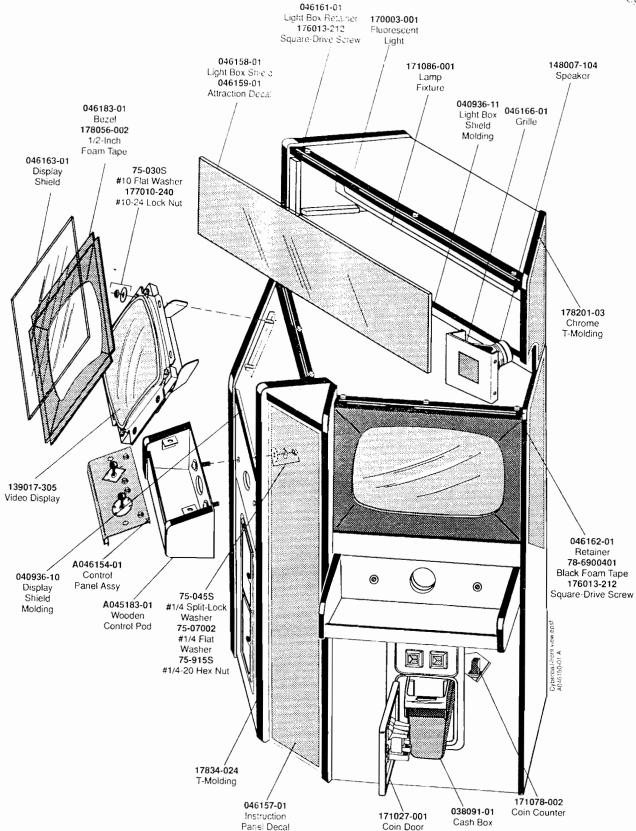
Figure 4-1 Cabinet-Mounted Assemblies, Front View A046150-01 B
