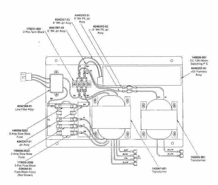
Figure 4-4 Power Supply Assembly A046211-01 A
