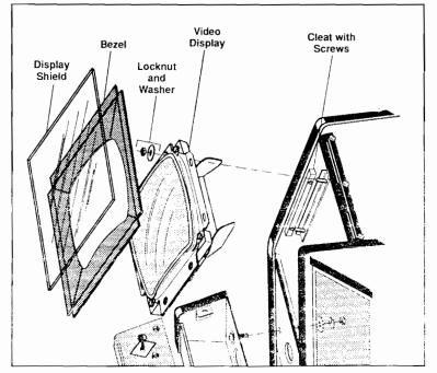
Figure 3-2 Removing the Video Display
