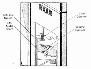
Figure 1-1 Control and Switch Locations
