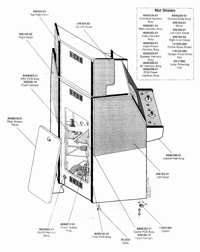
Figure 4-1 Cabinet-Mounted Assemblies, Rear View A046150-01 B
