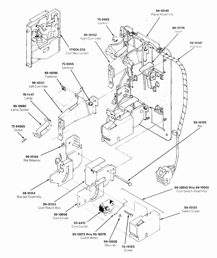
Figure 4-5 Coin Acceptors, Inc. Coin Door Assembly 171027-001 A
